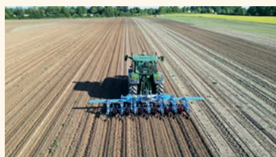
Active guidance of the tool to allow camera-free hoeing.
