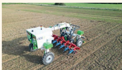
Tool holder used for independent sowing and hoeing.
