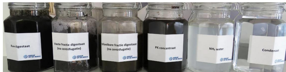
Figure 4: Raw digestate, solid fraction of digestate, liquid fraction of digestate, PK-rich concentrate, NH 3 water and condensate produced by Group op de Beeck
