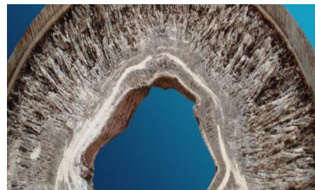
Figure 3: Struvite incrustations in pipes
